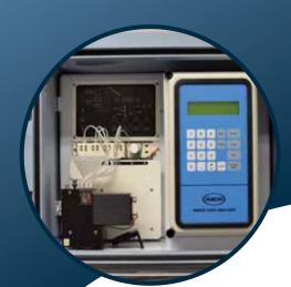
MPW's Mobile Silica Lab provides a fully automated, continuous analysis of silica levels in deionized product water. A manual sample may be taken from an easy-access lab faucet. The lab is climate controlled and includes an office for personnel.
